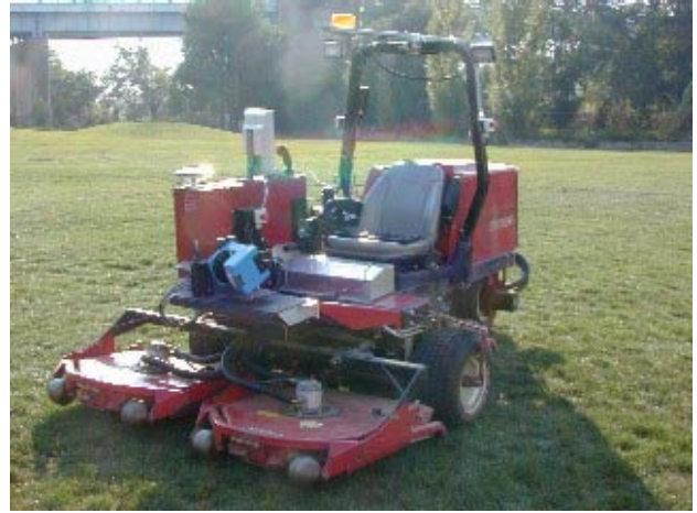
Figure 9: Mobile robot test platform is a retrofitted mower used for sports fields and golf courses.
