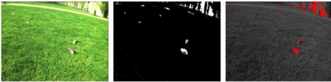
Figure 5. Color-based background filter. The model learns the appearance of grass based on its color (left), allowing uniquely colored objects to be segmented (center) and overlaid on the original image (right).
