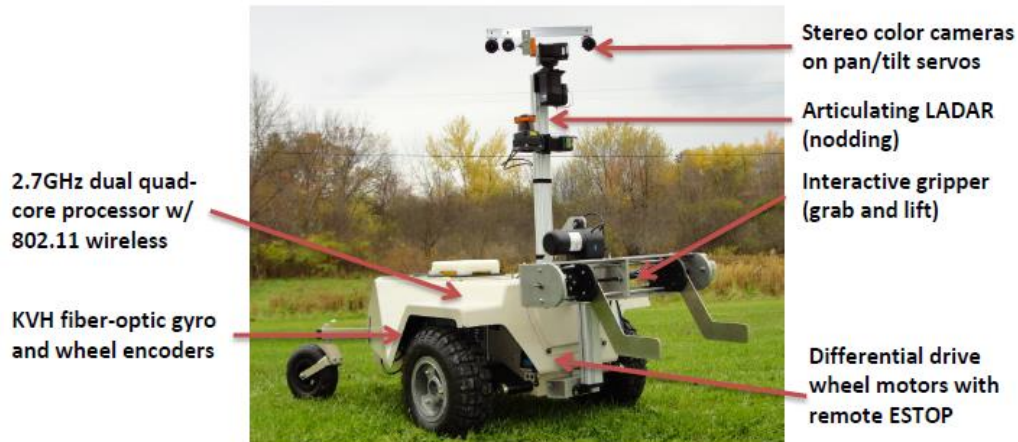
Figure 2. Neya's CANINE robot includes a mobile platform, a sensor mast with articulated LADAR and color cameras, and a front mounted gripper for picking up and placing objects on the ground.
