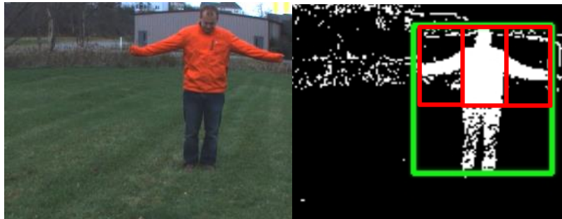
Figure 8. The operator detection filter uses background segmentation in combination with shape heuristics to identify static gestures. In the right figure, this the operator blob is outlined in green and the three vertical torso components are outlined in red.
