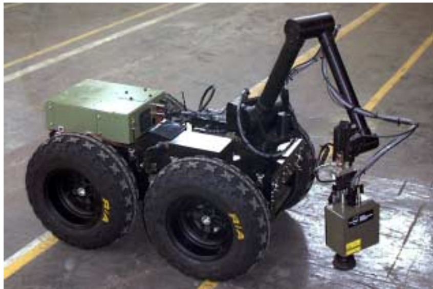
Fig. 4. Raman detector integrated on the ARES UGV
